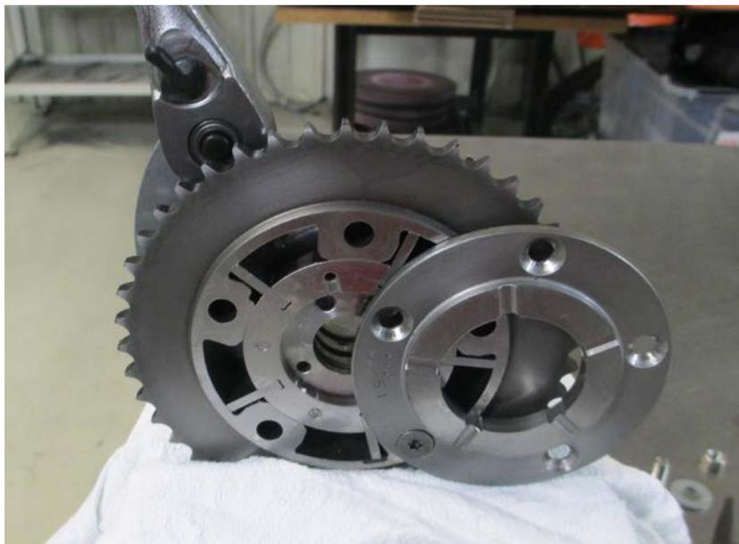
**Step 7:** Insert the cam phaser limiter block into one of the cam phaser control chambers; the slotted end goes in first.
