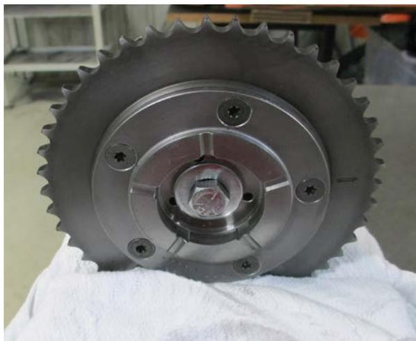
**Step 9:** Remove the cam phaser spring compression tool and the safety bolt assembly. The modified cam phaser is now ready for installation.
