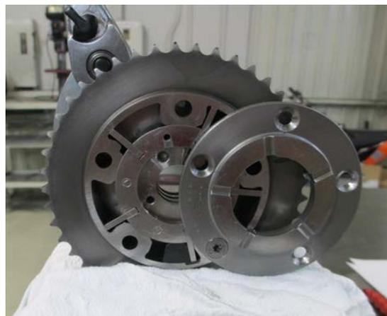
**Step 8:** Rotate the cover plate back over the control chambers and reinstall the safety bolt. Reinstall the cam phaser bolts, making sure to install the pin-bolt back into the correct position. Remember to torque the bolts to 85 in. lbs.
