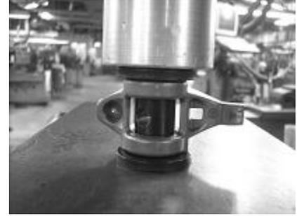
7. Picking up the rocker body, place the other included assembly washer beneath it. Ensure that the trunion fits through the center opening of the assembly washer.
