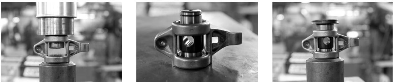
6. Drop in the trunion. Set the other bearing on top as flat as possible. Set 1 of the washers included with the kit on top of it, again letters facing outward. Press against washer so it slides around the trunion. Press only until light pressure is felt, this will start the top bearing install, ensuring everything stays lined up.
