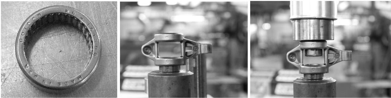
3. It is critical that the bearing be installed with the letters facing outward on both sides of the rocker arm!
