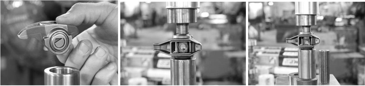
2. Gently press out the existing trunion using a ½ in. driver, being careful not to damage the rocker body. During the press out make sure that the die, driver and rocker arm remain straight. The factory trunion will unseat and come out relatively easily.
