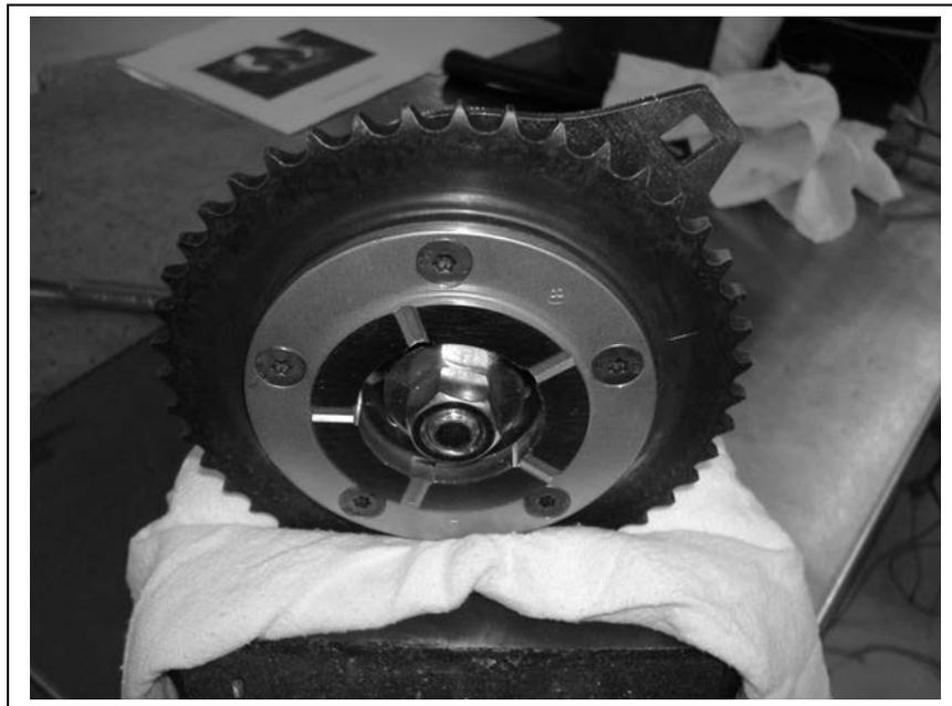
**Step 9:** Remove the cam phaser spring compression tool and the safety bolt assembly. The modified cam phaser is now ready for installation.
