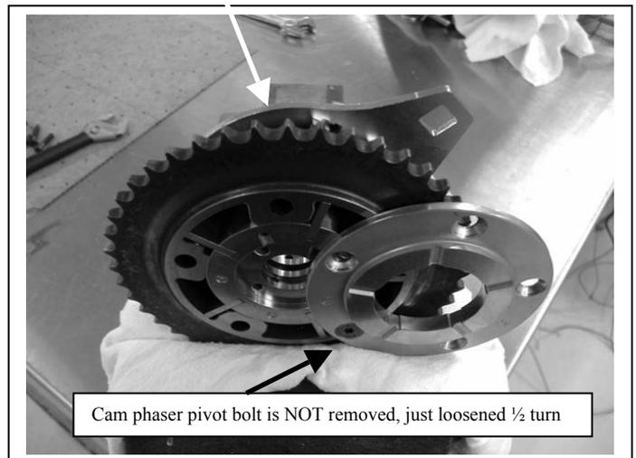
**Step 7:** Insert the cam phaser limiter block into one of the cam phaser control chambers; the slotted end goes in first.
