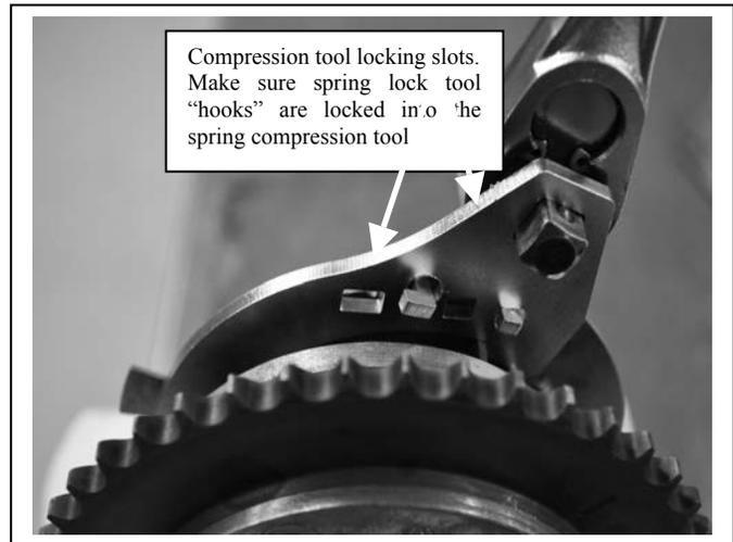
**Step 6:** Using the included TORX Plus bit, locate the pivot bolt and loosen it ½ turn. It is the first bolt located clockwise from the pin-bolt. Remember, DO NOT remove this bolt, just loosen it ½ turn. Remove the other four bolts and temporarily remove the safety bolt. Rotate the cover away to expose the phaser control chambers.
