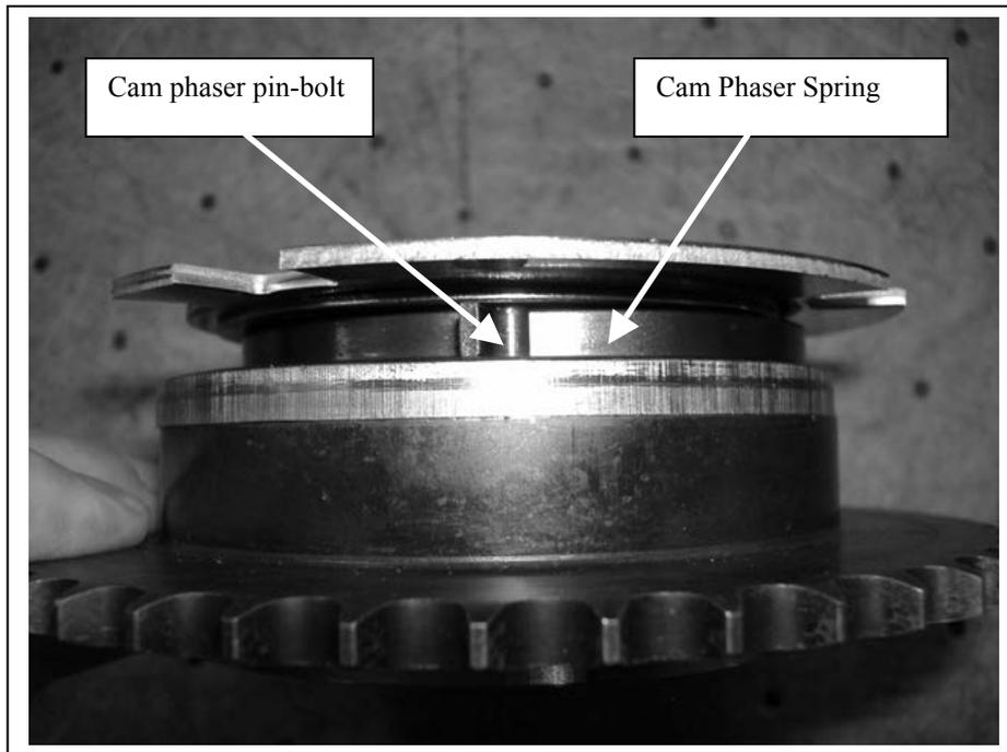
**Step 4:** Using a soft cloth to protect the cam gear, lock just the gear portion of the cam phaser in a vise. Do not over tighten the vise, use just enough force to secure the gear. Position the cam phaser in the vise with the pin-bolt at the 2-3 o'clock position, looking at it from the cam side. Take note that the first bolt located clockwise from this pin-bolt will not be removed. We will be using that bolt to pivot the cam phaser cover out of the way.
