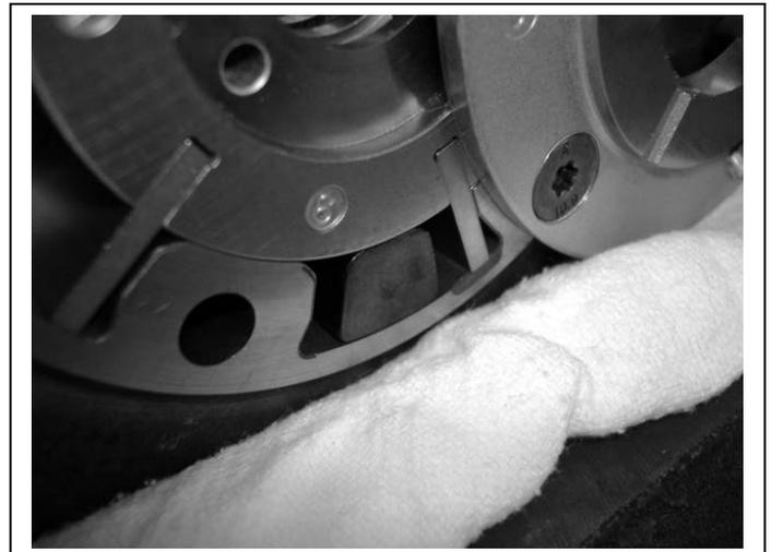
**Step 8:** Rotate the cover plate back over the control chambers and reinstall the safety bolt. Reinstall the cam phaser bolts, making sure to install the pin-bolt back into the correct position. Remember to torque the bolts to 85 in. lbs.
