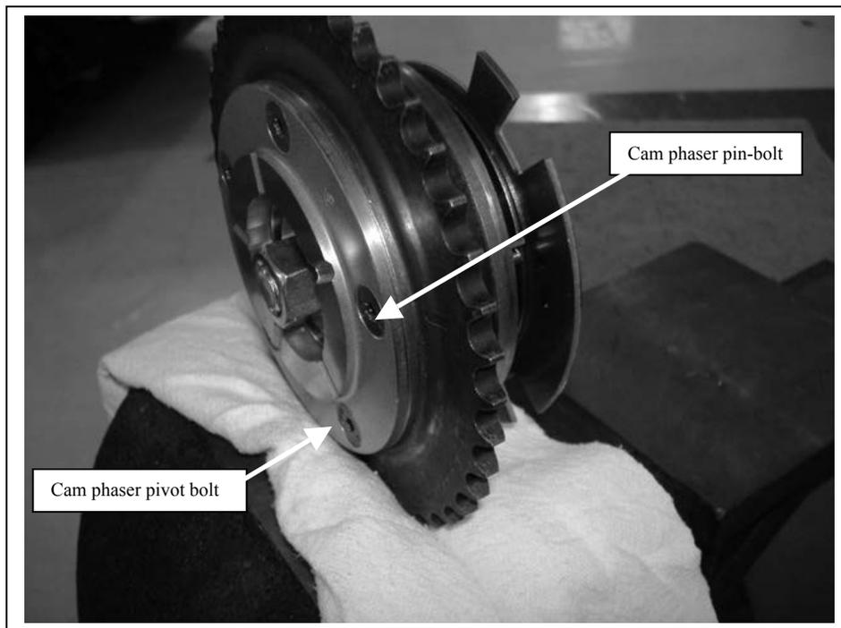
**Step 5:** Take the spring compression tool and hook it on the spring's L-bend where it contacts the pin-bolt; making sure the compression tool is centered on the phaser spring. Compress the spring by rotating the tool until the locking slots are visible, then insert the spring lock tool. Use the round holes for 2014 LT1 Applications.
