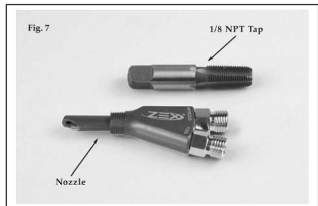
nozzle in a metal duct. Just drill a 11/32 inch hole where you want to mount the nozzle, tap the hole and install the nozzle. Once the nozzle is installed, place the appropriate tuning jets in the nozzle and attach the 2-foot long, -3AN hoses to the nozzle jet fittings and the nitrous management unit (Fig.6).
