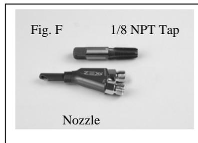
We've enclosed a tap (Fig. F) should you need to mount the nozzle in a metal duct. Just drill a 11/32-inch hole where you want to mount the nozzle, tap the hole and install the nozzle. Once the nozzle is installed, place the appropriate tuning jets in the nozzle and tighten the 2-foot long, -3AN hoses to the nozzle jet fittings and the Nitrous Management Unit. (Fig. G)
