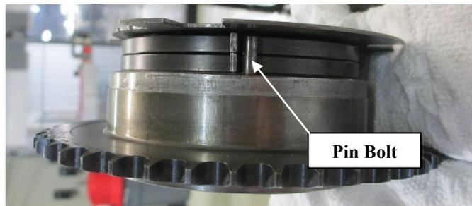
**Step 4:** Using a soft cloth to protect the cam gear, lock just the gear portion of the cam phaser in a vise. Do not over tighten the vise, use just enough force to secure the gear. Position the cam phaser in the vise with the pin-bolt at the 2-3 o'clock position, looking at it from the cam side. Take note that the first bolt located clockwise from this pin-bolt will not be removed. We will be using that bolt to pivot the cam phaser cover out of the way.
