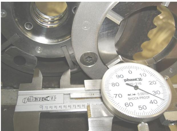
LT4 cam phasers have ~.935 in. chamber width
