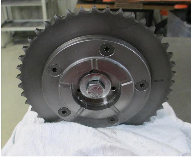
**Step 10:** Remove the cam phaser spring compression tool and the safety bolt assembly. The modified cam phaser is now ready for installation.
