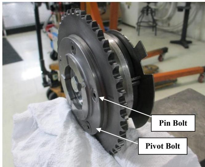
**Step 5:** Take the spring compression tool and hook it on the spring's L-bend where it contacts the pin-bolt; making sure the compression tool is centered on the phaser spring. Compress the spring by rotating the tool until the locking pin hole visible, then insert the spring lock pin.
