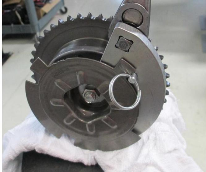
**Step 6:** Using the included TORX Plus bit, locate the pivot bolt and loosen it 1/2 turn. It is the first bolt located clockwise from the pin-bolt. Remember, DO NOT remove this bolt, just loosen it 1/2 turn. Remove the other four bolts and temporarily remove the safety bolt. Rotate the cover away to expose the phaser control chambers.
