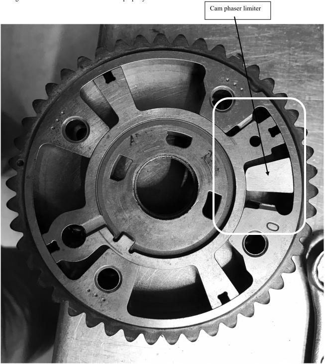
Step 7: Insert the cam phaser limiter block into the cam phaser control chamber as shown; the slotted end goes in first. It must go in this chamber as shown to function properly.
