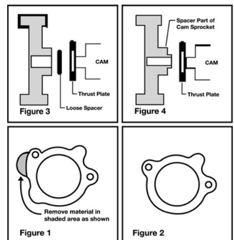
area shown in figure 1 will rub against the back side of the camshaft timing gear. The camshaft retaining plate should not come into contact with any part of the camshaft gear sprocket area. The only contact area between the camshaft retaining plate and the timing gear should be in the hub area.
