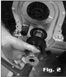
**Step 4:** Install crank pulley on crankshaft snout. Lubricate the bore and seal area of the crank pulley with COMP Cams® pro cam lube, part # 152. Use COMP® part #4789 crank gear installation tool and #4920 harmonic balancer installation tool to press pulley onto snout or a section of 2-1/4" o.d. x .375" wall aluminum tubing (fig. 2) as a driver. **Caution: Be certain that the crankshaft snout is not marred and that the crank hub seats squarely on the crank's shoulder step.**
