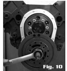
**Step 17:** The cam is now ready to be degreed per your requirements. If the engine is in the short block stage, you can set the No. 1 piston to Top Dead Center, and degree the camshaft as you would with any other timing set. Note that some engine builders prefer to advance cam an additional 1 to 1-1/2 degrees in order to compensate for belt stretch. When the degreeding process is performed on a long block, there is generally enough tension on the valve train to facilitate a direct setting.
