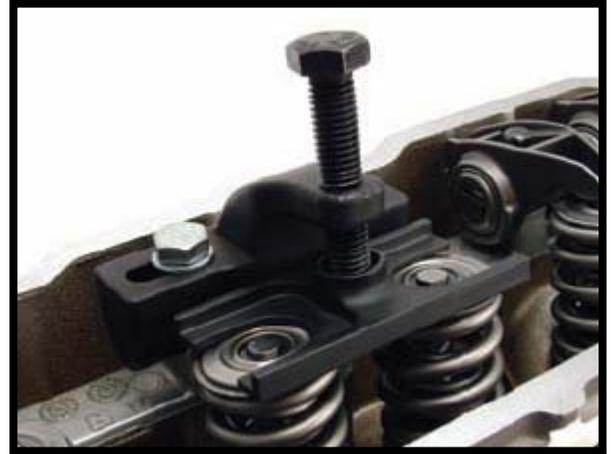
**WARNING: Never loosen the hold down bolts while the tool is under spring load!
