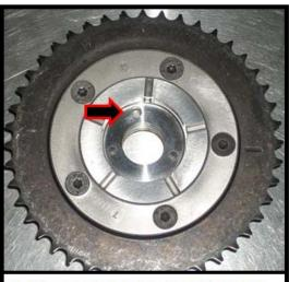
Find the correct hole for camshaft pin. The correct hole is larger and slightly oblong.
