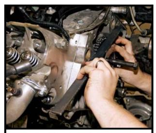
Use a straight edge to ensure phaser and timing chain do not protude from the block
